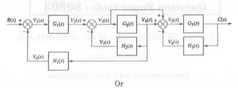
(b) Determine the transfer function for the signal flow graph using Mason Gain Formula.
